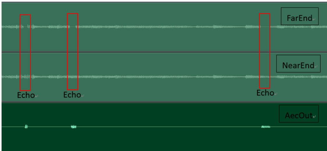
Figure 5: The Far-End signal is not fed in AEC when the echo appears (The result will be affected.)
