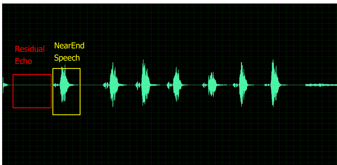
Figure 30: AEC digital output signal (AecOut). AEC mode is set as 15
