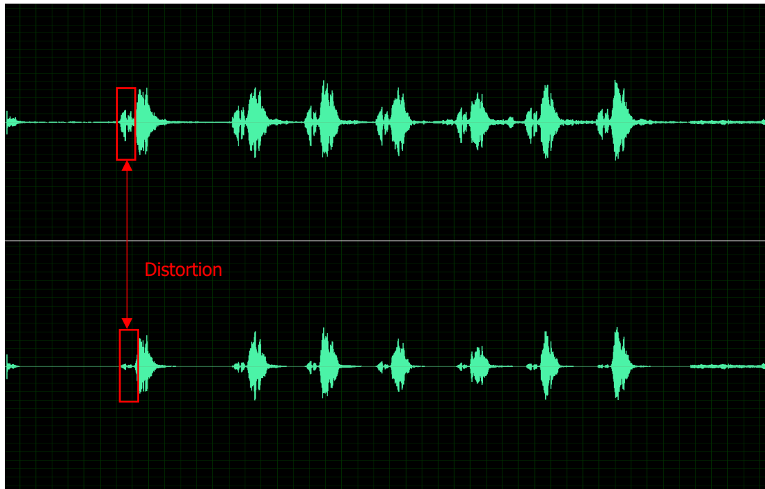
Figure 26: This figure shows the distortion when double talk, the power of near-end speech may decrease
