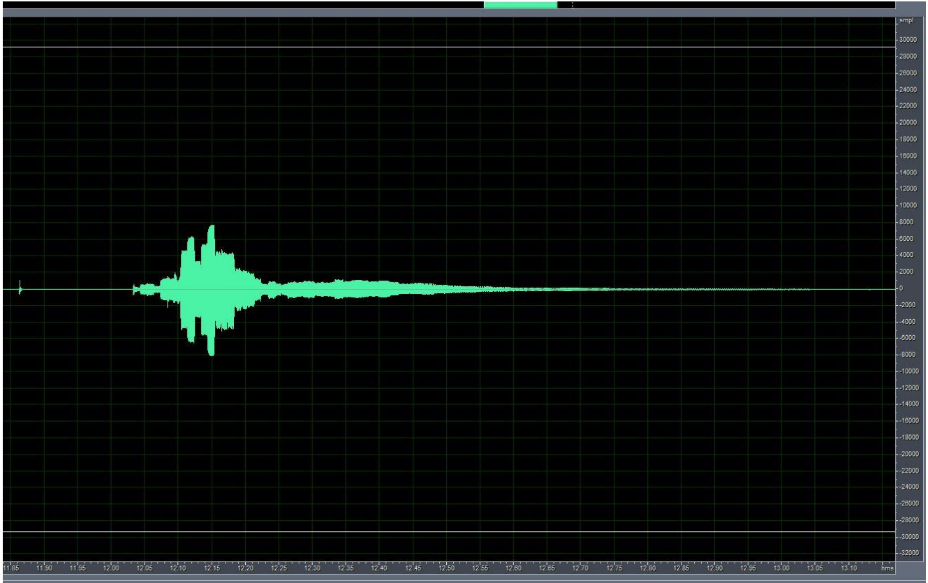
Figure 18: The acoustic echo when play out a sweep wave from speaker.
