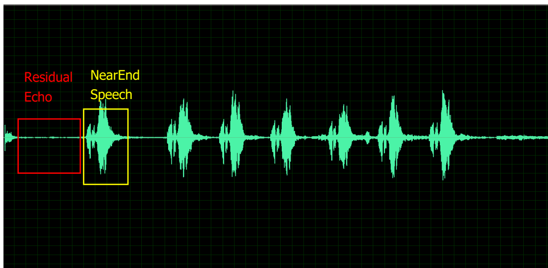
Figure 29: AEC digital output signal (AecOut). AEC mode is set as 4
